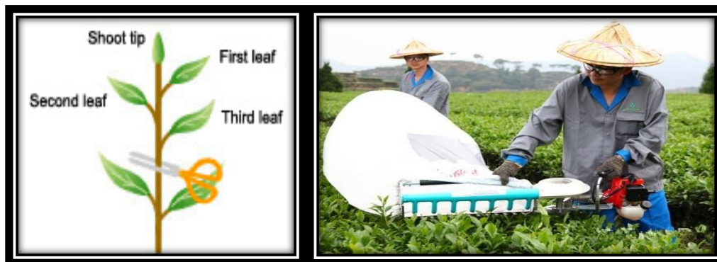
Fig. 4: Picking of green tea leaves with the help of tea picking machine
